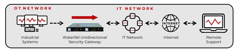
The Waterfall RSV uses an internal, hardware based, unidirectional fiber optic link to replicate the contents of server and workstation screens from industrial networks to enterprise networks and the Internet, in real time. The Unidirectional hardware makes it physically impossible for data to flow from the corporate network towards the industrial network, eliminating any threats of cyber-attacks, incoming malware or human errors.
