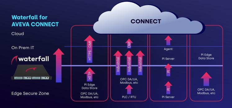
Waterfall Unidirectional Security Gateways can securely transfer data from industrial systems to AVEVA Connect from PI Edge Data Stores, OT industrial devices, and PI Servers.
