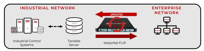
Waterfall for Tenable Update enables seamless vulnerability and security management updates for operations networks while eliminating the risk of remote-control attacks, malware, and other attacks on protected OT networks. The Waterfall for Tenable Update connector supports both Tenable SecurityCenter and Tenable Nessus.
