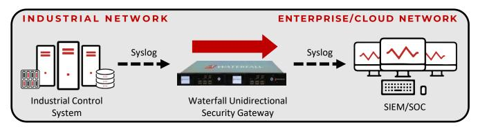
Central security monitoring is focused on events and alerts encoded as Syslog messages. Waterfall for Syslog is a standard Syslog server on a protected industrial network, gathering Syslog messages from that network. Syslog alert content and metadata are forwarded through Unidirectional Gateway hardware. On the external network, new Syslog alerts are formulated and sent to a central enterprise or cloud-based SIEM or SOC installations without risk to operations.
