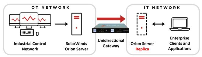
Waterfall for SolarWinds Orion is part of the Waterfall Unidirectional Security Gateway family of solutions. The Orion server replication software queries the Orion server on an industrial network for current data, sends that data across Unidirectional Gateway hardware to an enterprise network, and uses the data there to populate the enterprise Orion server. Enterprise users can use the visualization, monitoring and analysis capabilities of the enterprise server to access and manipulate OT data.
