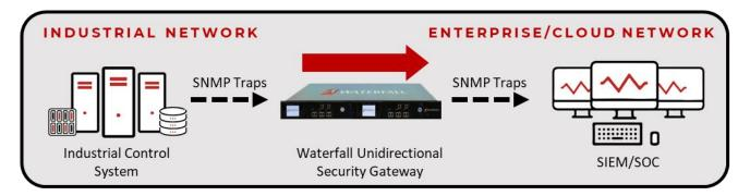
Waterfall for SNMP receives SNMP traps according to user-configured rules. Trap content and metadata are forwarded through Waterfall's Unidirectional Security Gateway hardware to one or more central Network Management Systems (NMS) or Security Information and Event Management (SIEM) systems, most often in a Security Operations Center (SOC).
