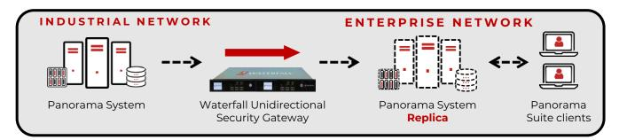
Waterfall for Panorama enables safe configuration file, database and other transfers from OT to IT networks while securing OT networks against cyber threats from enterprise networks. The solution can act as a file transfer client, pulling files from the operations network and replicating them to machines on IT networks. Waterfall's sophisticated file filtering ensures that only approved file types with set characteristics are made available on enterprise networks.
