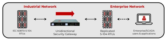
The Waterfall for IEC 60870-5-104 connector is part of the Waterfall Unidirectional Security Gateway family of products. The connector polls RTUs and other 60870 devices on industrial networks in real time, sends that data across the Unidirectional Gateway hardware, and emulates the 5-104 devices to enterprise users and applications, such as enterprise historians.
