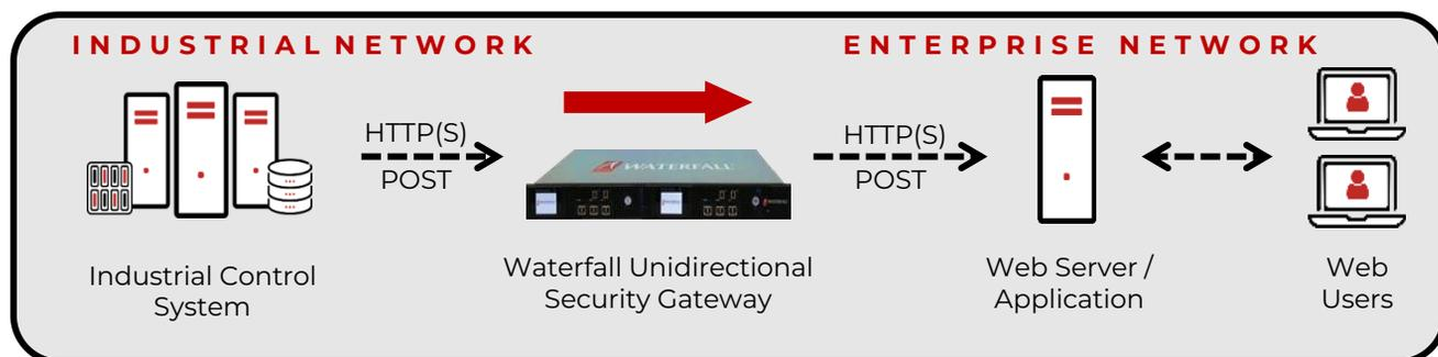
Waterfall for HTTP(S) is part of the Waterfall Unidirectional Security Gateway family of products. On the industrial network, the connector is most often an HTTP(S) web server, receiving POST requests from industrial systems. On the enterprise network, the connector is most often an HTTP(S) client, posting files and other content to enterprise web applications and servers.
