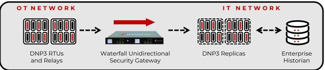
The Waterfall for DNP3 connector is part of the Waterfall Unidirectional Security Gateway family of products. The connector polls RTUs and other DNP3 devices on industrial networks in real time, sends that data across the Unidirectional Gateway hardware, and emulates the DNP3 devices to enterprise users and applications, such as enterprise historians.
