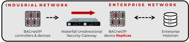
The Waterfall for BACnet/IP connector is part of the Waterfall Unidirectional Security Gateway family of products. The connector polls controllers and devices on industrial networks in real time, sends that data through the Unidirectional Gateway hardware, and replicates the BACnet/IP devices to enterprise users and applications, such as enterprise historians.
