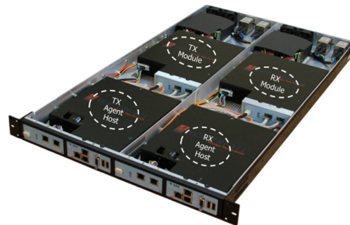
Figure (1): Waterfall’s Modular Unidirectional Gateway Hardware Architecture
